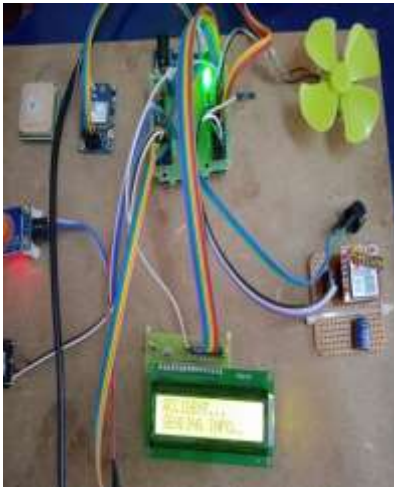
Fig 14: Sensors and ESP32 CAM interfaced with the Arduino
